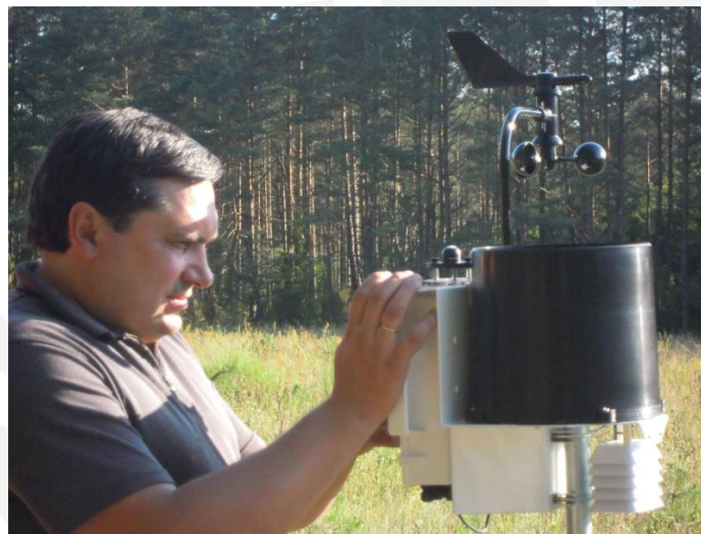
5 pav. WatchDog 2700 weather station (Spectrum Technologies Inc.) (SLĖNIS NEMUNAS).
