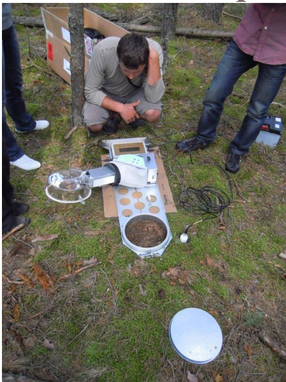
4 pav. ACE soil CO 2 exchange system (ADC BioScientific LTD) (SLĖNIS NEMUNAS).
