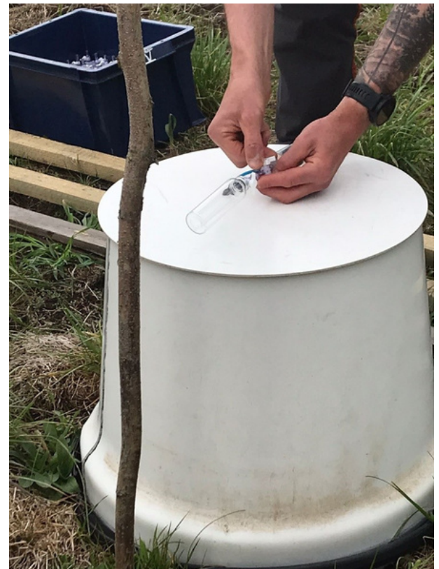
Figure 1. Taking a gas sample.
