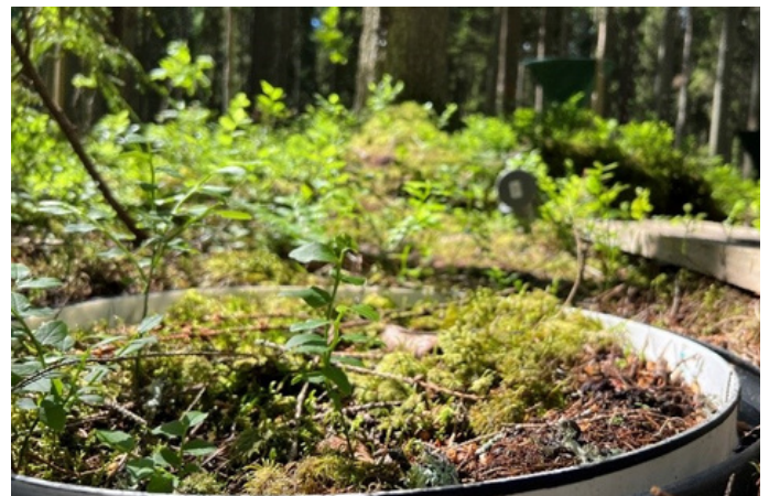
Figure 1. Ring for the SEG fluxes collecting chambers.
