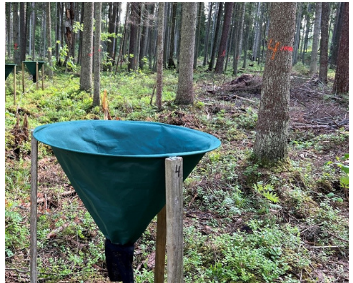
Figure 3. Litter trap for small size litter.
