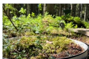
Figure 1. Ring for the SEG fluxes collecting chambers.
